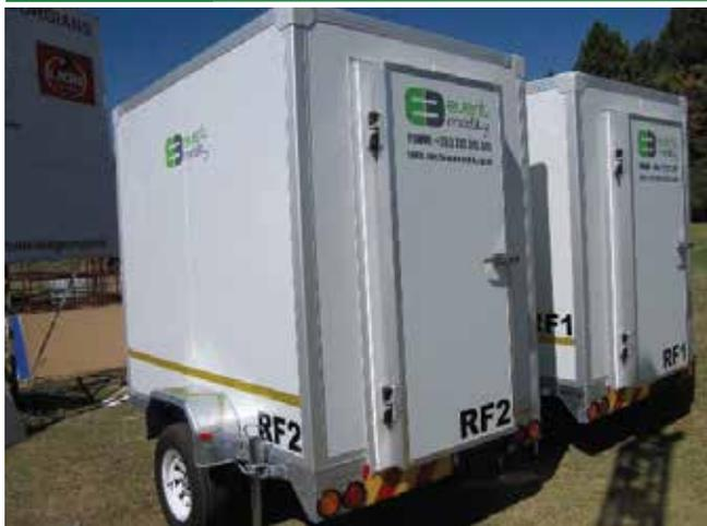
Event Mobility offers refrigerated units which are ideal for onsite catering services and bar services. The units run off 15amp power and are able to be cooled down to 1 degree Celsius. The units have internal stainless steel shelving which assist in optimising space inside the trailer.
